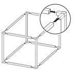
Don't worry if the frame seems a little wiggly or loose. Make sure all the tubes are pushed into the hubs. When the vinyl covering is put on, it will compress the frame and tighten it up.
