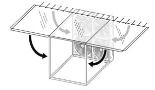
After you have secured the hook-and-pile fasteners along the edges, stretch the bungee cord connections into the fan wall notches. Start with the center top and work your way across and down to the bottom corners.
