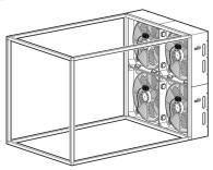
The vinyl covering easily picks up dirt, so make sure the floor is clean before unrolling the vinyl covering on the floor. One of the long edges has three strips of hook-and-pile fasteners on it. Place the covering on top of the frame with the hook-and-pile fasteners pointing down towards the floor. Roll the center top hook-and-pile fastener flab over the front of the frame and attach it to the hook-and-pile fastener on the inside of the frame. Do the same with the sides of the wind tunnel.
