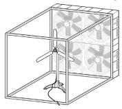
The fans running at high speed are noisy and windy. You can either leave them on during wind turbine performance testing, or shut them off between tests. Use the switch on the power cord to turn all the fans off and on at the same time.
