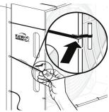
Plug all the fans into a power strip. Fans can be individually adjusted at the motors, although we recommend using the high setting. The average wind speed is approximately 3.6 m/s at a distance of 30 cm from the opening.
