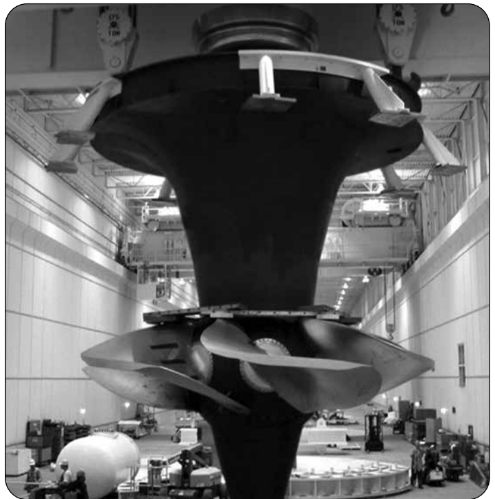
This fish-friendly turbine has openings large enough for fish to pass through.
