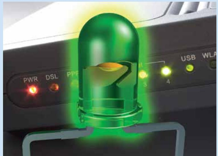
electricity flows. If it is connected the wrong way around, it will remain dark. LEDs have a few important advantages over conventional light bulbs: They use much less electricity for the same amount of brightness, and have a much greater life span.
