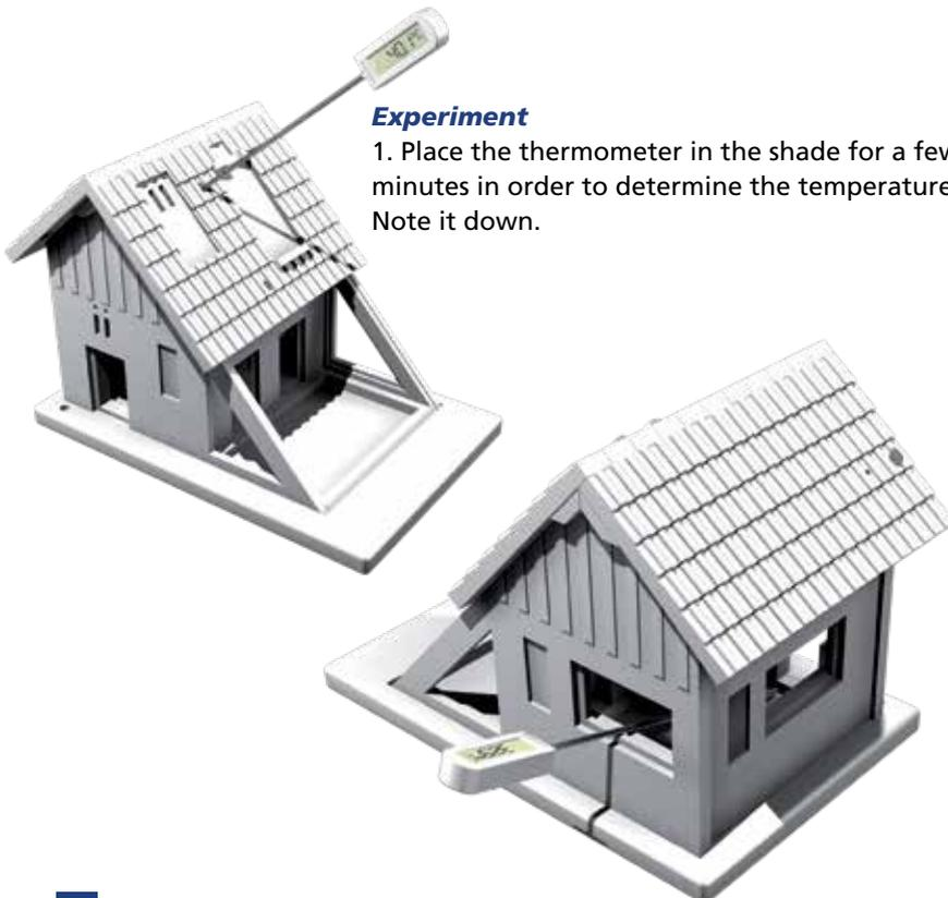
2. Set the house in the full sun with its windows open. Do not mount the transparent pane on the solarium annex. Insert the thermometer into the hole at the top of the roof, so that the sensor is in the apex of the house.
