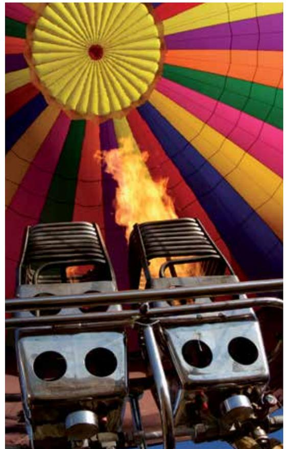
*The air inside a hot air balloon is heated with large burners in order to make it rise.*
