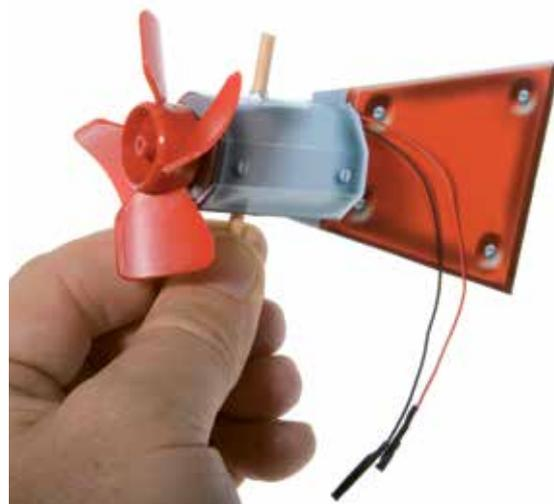
4. Insert the long dowel through the large opening at the side of the roof and into the hole in the base platform. The hole in the dowel must be pointing up. Now insert the short dowel with motor, propeller, and steering vane into that hole.
