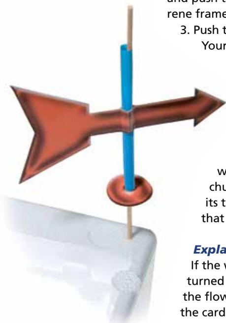
pressure makes it rotate until it has the smallest possible surface area turned toward the wind. Then the tip is pointing in the direction from which the wind is coming.
