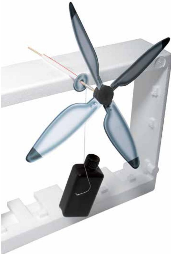
pieces from the die-cut sheet, and tape each one onto a short wooden stick. Remove the short rotor blades from the disk and replace them with the long ones. Push them in firmly so they don't slip out. Adjust the cardboard pieces to the optimal angle.
