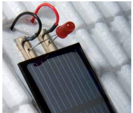
2. Position the Power House so that sunshine hits its solar cell. The LED lights up and the motor runs.
