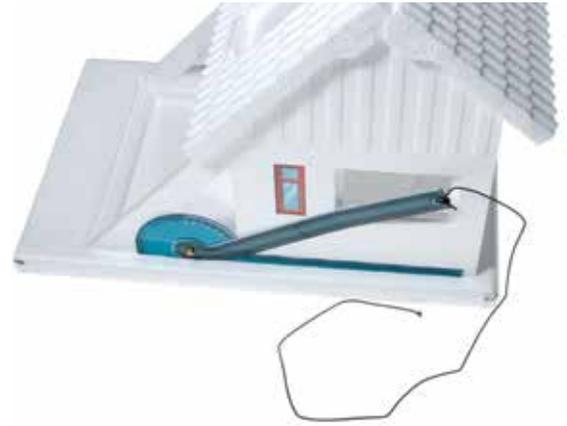
2. Open the two large windows and cut a section of yarn about 1 m in length. Tie one end to the angle gauge pointer, and the other end to a flashlight. Have an assistant shine the flashlight onto the house at a 60-degree angle, on the side of the house with the living room window. You will be able to tell by looking through the side window whether the flashlight beam is lighting the floor.
