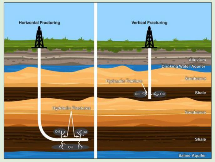
fractures in the shale rock, which contains the oil or gas. Sand from the fracking fluid holds the fractures open, which allows the oil or gas to flow into the well and be recovered by the crew at the earth's surface. This entire process of creating an operational fracking site takes about three to five months. The well can then potentially be used to produce oil or natural gas for the next 20 to 40 years.<sup>3</sup>
